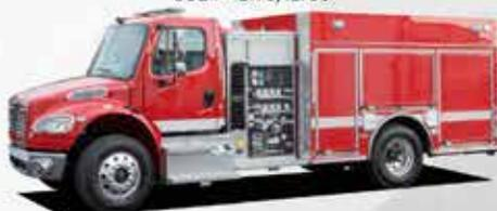
FREIGHTLINER M2-106 CHASSIS | SEATS TWO 1250 GPM | 152" BODY | 360HP CUMMINS
