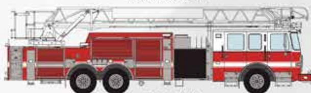
ENFORCER CHASSIS | 500 GALLONS | 2000 GPM WATEROUS 70" CAB | SEATS SIX | TAK-4 IND. FRONT SUSPENSION
