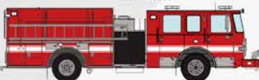
SABER CHASSIS | 70" CAB | LOW HOSEBED | LAP DOORS SEATS SIX | 1500 GPM | 510 HP | 152" BODY
