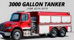
FREIGHTLINER M2-106 CHASSIS | 1000 GPM 10" NEWTON REAR & SIDE DUMPS | DETROIT DD8 375 HP
