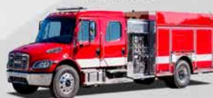
FREIGHTLINER M2-106 CHASSIS | SEATS FIVE 1250 GPM | 152" BODY | 360HP CUMMINS
