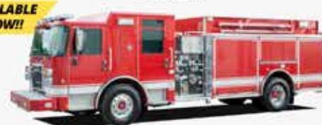
SABER CHASSIS | 70" CAB w/ 10" RAISED ROOF 10" NEWTON REAR DUMP | 1500 GPM | CUMMINS 450 HP
