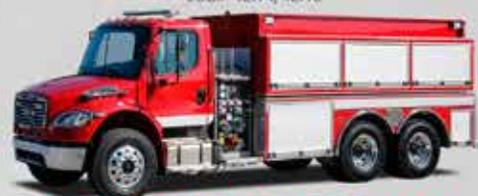
FREIGHTLINER M2-106 CHASSIS | 1000 GPM 10" NEWTON REAR & SIDE DUMPS | DETROIT DD8 375 HP
