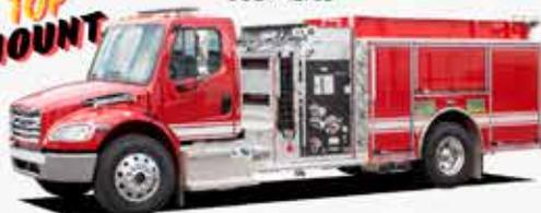
FREIGHTLINER M2-106 CHASSIS | TOP MOUNT CONTROLS 1250 GPM WATEROUS | CUMMINS 360 HP
