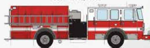
SABER CHASSIS | 70" CAB | LOW HOSEBED | ROLLUP DOORS | SEATS SIX | 1500 GPM | 510 HP | 145" BODY
