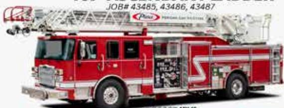
ENFORCER CHASSIS | 500 GALLONS | 2000 GPM WATEROUS 70" CAB | SEATS SIX | TAK-4 IND. FRONT SUSPENSION
