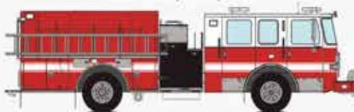
SABER CHASSIS | 70" CAB | LOW HOSEBED | LAP DOORS SEATS SIX | 1500 GPM | 510 HP | 145" BODY
