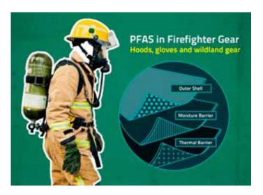
A firefighter's protective clothing is composed of three distinct layers made of different textiles. In response to concerns about the gear possibly exposing firefighters to PFAS chemicals—several of which have been linked to cancer—NIST researchers investigated the presence of the chemicals in textiles used to make the layers. This latest study analyzed hoods and gloves worn in structural fires as well as protective clothing worn to fight wildfires. Credit: B. Hayes/NIST
