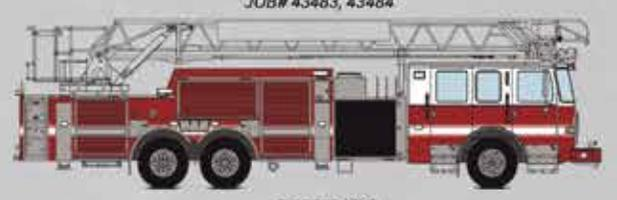
ENFORCER CHASSIS | 500 GALLONS | 2000 GPM WATEROUS 70" CAB
