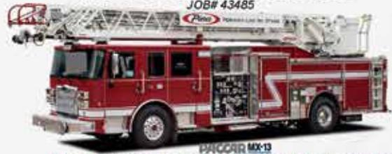
ENFORCER CHASSIS | 500 GALLONS | 2000 GPM WATEROUS 70" CAB
